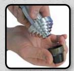
Snap hollow punch cutting head onto mandrel/handle.
